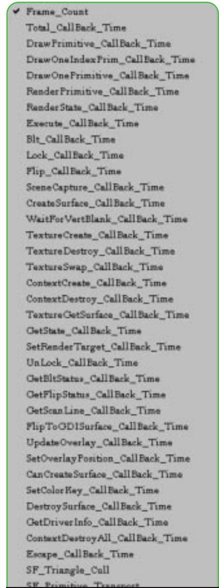
FIGURE 3. A partial list of the driver's counters that you can watch through OA.
