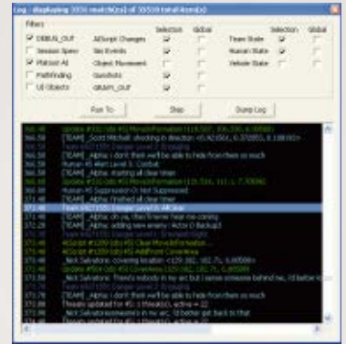
FIGURE 3 The Gravy message log can be filtered by information type and the selected object. The log can be dumped to a text file for search operations.
