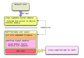
Accessing the device's internal memory Getting to debug firmware code
