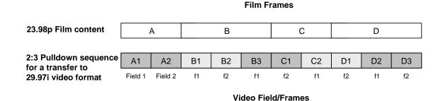
This 2:3 sequence shall be respected not only for transfers on telecines but also for frame rate conversions performed with any other system (standard converters, non-linear editing systems, etc.). It will ensure a fluid perception of movements.
