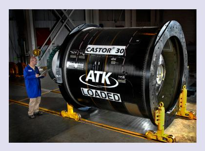
The Antares second stage is powered by a CASTOR 30 solid rocket motor produced and tested at ATK facilities in Utah. The CASTOR 30 motor is based on the proven CASTOR 120 motor that has been utilized in more than a dozen space launch vehicle missions.
