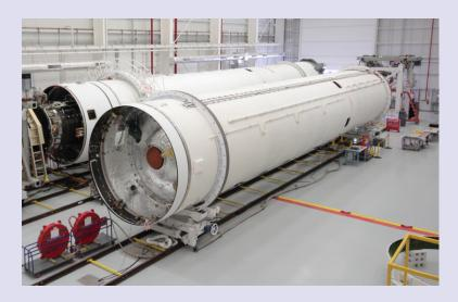
The Antares stage one structure is designed and manufactured by the Yuznoye Design Bureau of the Ukraine based on Zenit launch vehicle heritage. The stage one core is shipped to the Port of Wilmington, Delaware and transported by truck to the Wallops Island, Virginia launch site for integration with the engines, upper stage avionics and fairing.
