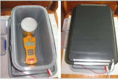
This is a photo of a basic built lead shielded, but without copper inner liner test chamber, with 15mm walls.
