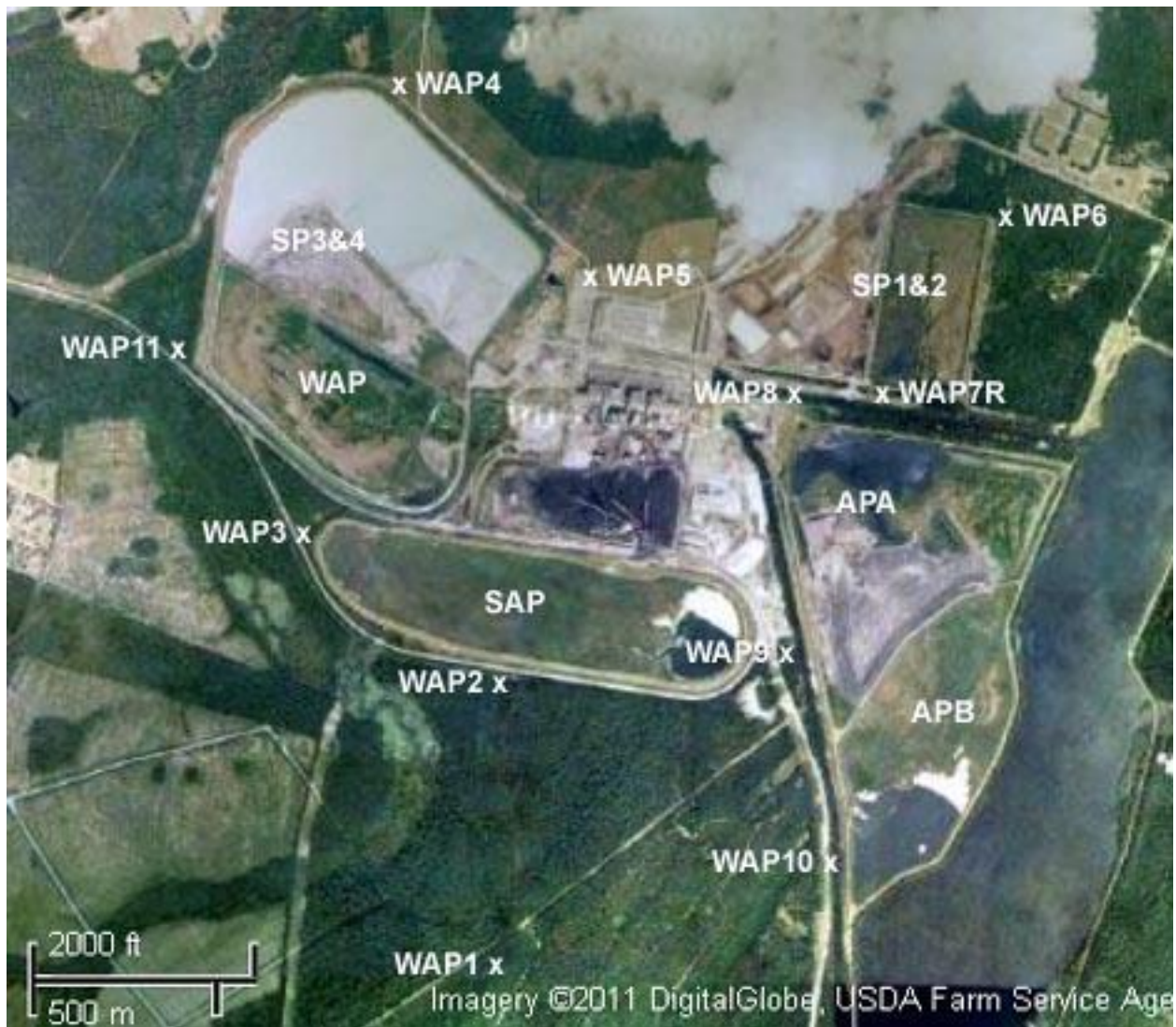
Winyah Generating Station Ash and FGD Ponds and Monitoring Well Locations. Ash Pond A (APA), Ash Pond B (APB), West Ash Pond (WAP), South Ash Pond (SAP), Slurry Ponds (SP1&2 and SP3&4); Monitoring Wells WAP1 to WAP11.
