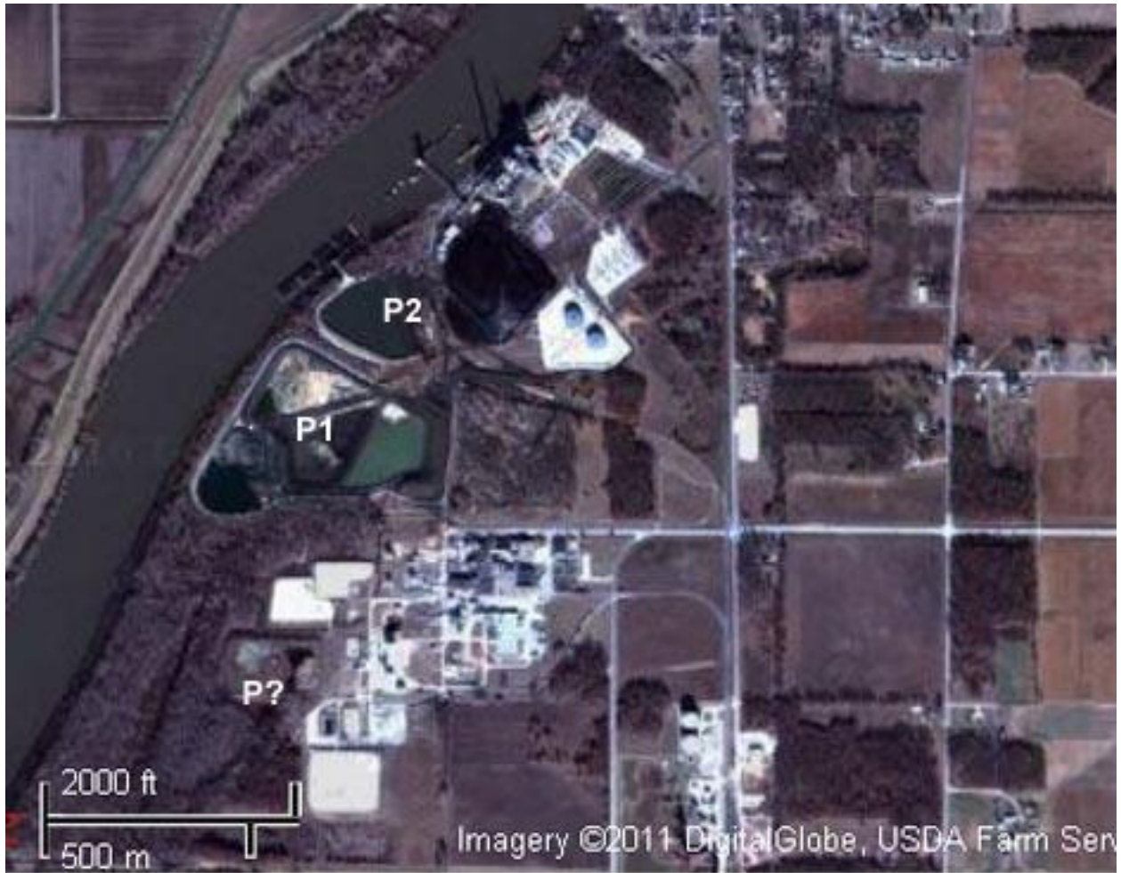
Meredosia Power Station Ash Ponds, Meredosia, IL. P1 = Active Fly Ash Pond, P2 = Active Bottom Ash Pond.
