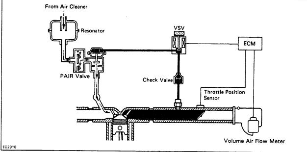
To reduce HC and CO emissions, this system draws in air into exhaust ports to accelerate oxidation, using vacuum generated by the exhaust pulsation in the exhaust manifold.
