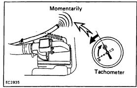
(c) Race the engine and quickly close the throttle valve. Check that a bubbling noise stops momentarily.
