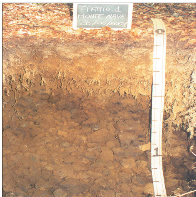
Andosols of the western slope of Mount Etna in Sicily, Italy formed by lava flows with tephra – fragmented rocks deposited by pyroclastic flows from an erupting volcano (CD).
