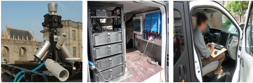
(a) To the roof, instruments of measurements have been mounted on a mast. (b) At the back, a unit of secure data storage and a power station control system have been fixed. (c) At the passenger side, a on-board computer has been installed.
