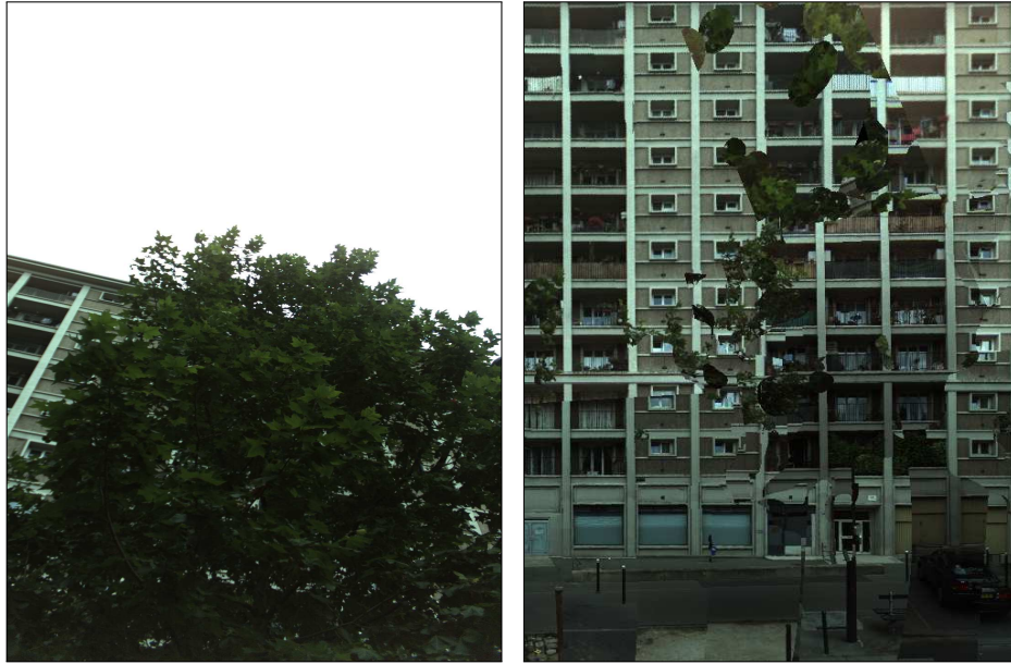
(a) Frontal image facing the facade top strongly occluded by the foliage of a tree. (b) Multiview reconstructed occlusion-free facade texture
