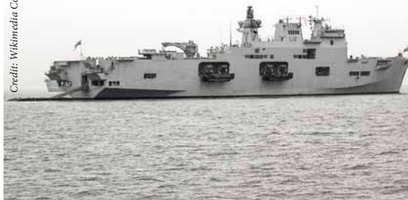
HMS Ocean at the 2005 International Fleet Review, showing landing craft on davits and stern ramp deployed.
