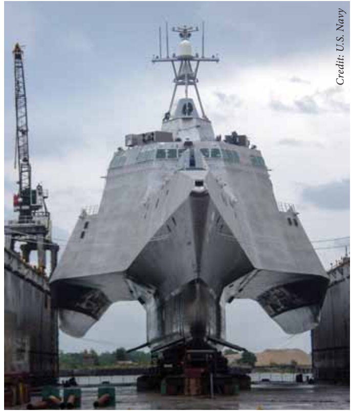
The Littoral Combat Ship pre-commissioning unit Independence (LCS 2) is the second ship in a new design of next-generation combat vessel for close-to-shore operations. It has a crew of less than 40 sailors, can reach a sustained speed of up to 40 knots and can accommodate two SH-60 Sea Hawk helicopters.
