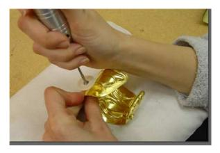
**Step Four:** The bracelet is shaped over a mandrel and the bezels are soldered on. The height of each bezel is adjusted by sanding the top.
