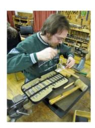
working end is roughened by sanding, or filing in order to grip and move the metal easier. Shapes may vary, but a basic set should at least consist of an oval, round, square, tear drop, rectangular and half-round punches.
