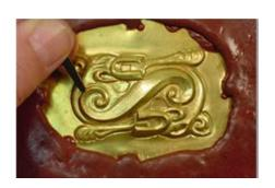
Tools should be made of the smallest appropriate size steel stock. The most commonly used sizes are those between ¼ " and 1/8 " ( both round and square) cut into 4" to 4 ½ " lengths. Shape the tool roughly on the 36 grit grinding wheel, then continue to work by files, 400 and 600 grit sand paper, and at the end polish with steel compound. Polishing will eliminate even the slightest imperfections.
