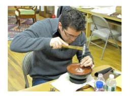
weight. For chasing large pieces, a large cast iron frying pan can be used. You may also build a wood frame with the desired dimensions and attach it to a piece of plywood. Melt the pitch in a separate container and pour into the frame. A minimum of 3" layer of pitch is necessary.
