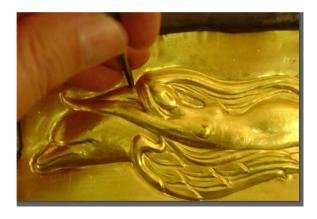
**Step Three:** After raising the relief, the metal is annealed and put face up in the pitch for final chasing.
