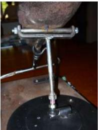
On top of the shaft we placed a sling shot shaped piece of  $1/4 \ge 1/2$  flat bar. There are holes drilled in each end to accommodate a 1/4" bolt. We then welded a piece of tubing or small pipe to the bottom of the arm rest. The arm rest is attached to the shaft by running the bolt through the sling shot and tubing to create a hinge.
