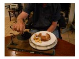
Above is a picture of Glen demonstrating how it works. His right arm is positioned on a rest that is mounted to a  $12^{\circ} \times 18^{\circ} \frac{3}{4}^{\circ}$  plywood board. There are three directions of movement required that have to attained in order to eat. We will explain these as we proceed. There is also a "lazy susan" below the plate to allow him to rotate his plate if he needs to.
