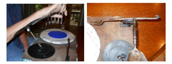
The next question was how do we attach the eating utensils? We wanted a way to be able to quickly attach a fork or spoon. Glen is right handed, so we decided to weld a <sup>1</sup>/<sub>4</sub>" socket extension to the left side of the Harbor Freight handle. On the other side we forged a "curl" to prevent his hand from sliding off the rest. These components are essential to form a hand rest and
