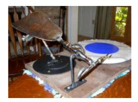
The arm rest was made from 18 gauge sheet. The pattern was cut "to fit" slightly less than the length of Glen's arm – wrist to elbow. A swage block was used to put the dip/curve in it. Note that both sides of the back end are flared out so that when pressure is put on it the users arm will not slide off. The flared part is important to assist in the turning movement.
