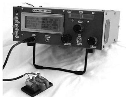
Figure 3 — We built this portable PSK unit around 2000. It was too complex and expensive, with separate boards for DSP and control processing. It did include a novel CW user interface.
