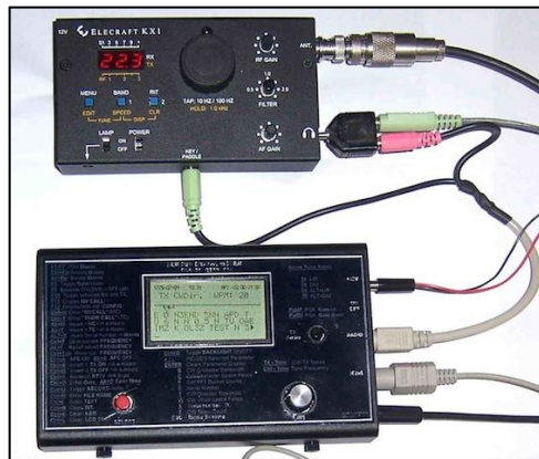
Connections from the NUE-PSK Modem to the Elecraft KX1 CW Transceiver
