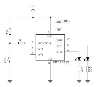
The LED on GP1 is initially turned on, and then when the pushbutton is pressed, the LED is turned off (reducing power consumption) before placing the PIC permanently into sleep mode (effectively shutting it down).
