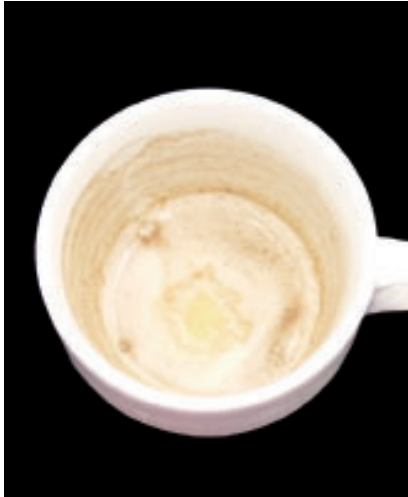
Yellow-brown residues (e.g. tea, coffee); removable; detection: chlorine bleach (RB test kit)
