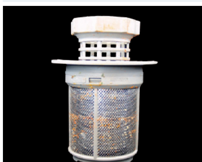
Deposits of soils or grease in outlet areas, e.g. filters
