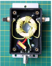
Transformer type: 50 ohms to 800 ohms (1:16) balun. **Balun details are on separate document at the web page.** Components were fitted with hot-glue into the ABS box. 6.3mm AMP terminals are for connecting antenna wires. BNC connector with flange for 50 ohms coaxial feed gable. The box was finally potted with beeswax. In this case we used three ferrite tubes as choke balun. Tubes were assembled over the coaxial.
