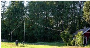
NVIS inverted-V with parallel vertical wires:
