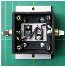
800 Ohms low-inductance resistor is fitted into ABS box. Resistor type is 2x **MP930-400, 400R 30W**, (Elfa). Box is fitted into 3mm aluminum sheet and then to profile heatsink. 6.3mm AMP terminals are for connecting the antenna wires. The box was finally potted with beeswax.
