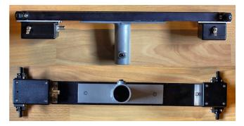
Terminal & balun boxes are fitted into heatsink (20x80x450mm). Horizontal wire-spacing is 450 mm. Antenna mast is free-standing 50/38mm steel tube mast, top 8 meters. Mast & antenna survived last winters storm, gusts over 30 m/s.
