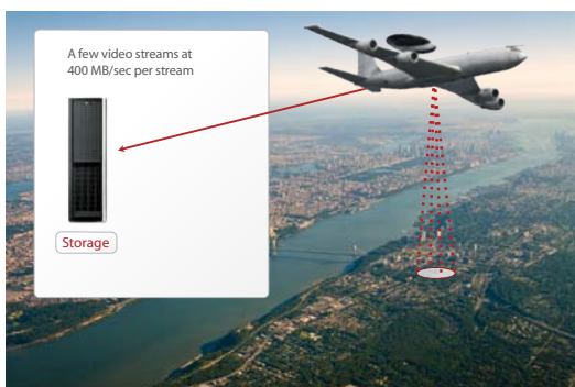
Surveillance Area and Camera Resolution Limited by bandwidth of backend storage
