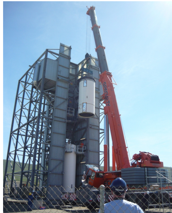
Figure 5-4: Minotaur IV Stage 2 Lifting Operation Using a Portable Crane
