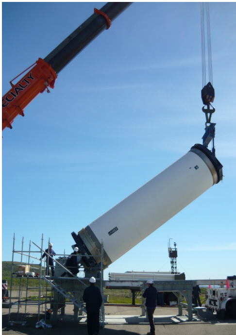
Figure 5-3: Minotaur IV Stage I Lifting Operation Using a Portable Crane
