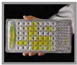
Total coliforms (and E. coli ) on Colilert in Quantitray format
