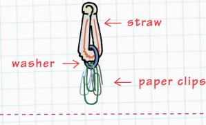
**3. Test.** Place the diver into a container of water and test its buoyancy. Keep redesigning until the diver "hovers" in the center of the container of water.
