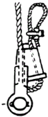
Figure 35.27. Dead-Ending Rope in a Socket.
