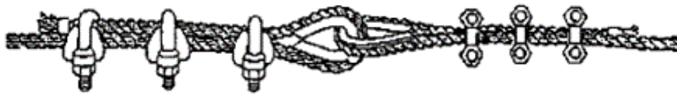
Figure 35.26. Joining Wire Ropes.
