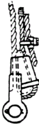
Figure 35.27. Dead-Ending Rope in a Socket.
