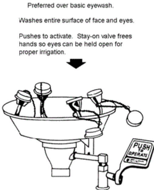
Figure 19.7. Wall-Mounted Permanent Eye and Face Wash.
