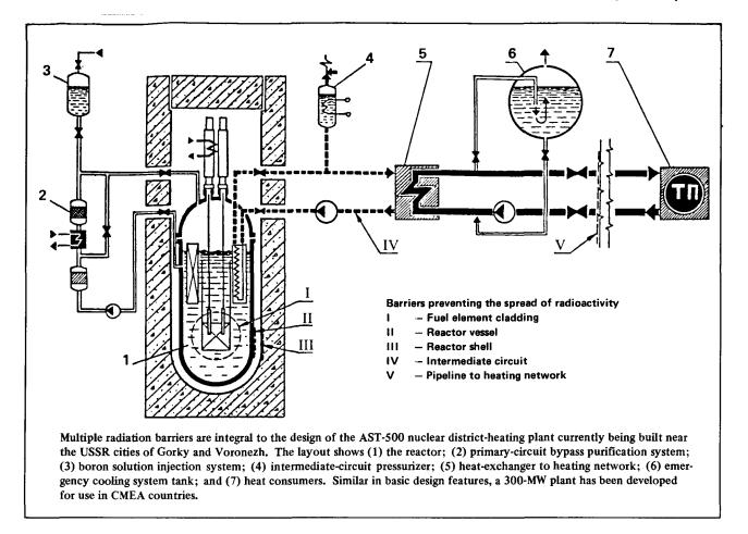
• A three-circuit design for heat removal from the reactor with an intermediate separating circuit, inside which pressure is lower than in the heat network, precludes escape of radioactive products from the reactor to the customer through leaks in the heat-exchange surfaces.
