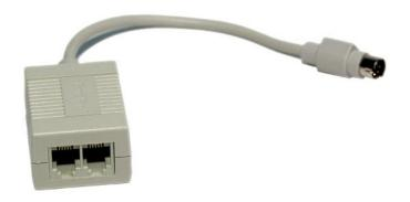
• Two LocalTalk connectors are REQUIRED. One of these connectors must be plugged into the Asanté Talk via the attached din-8 cable. The other must be plugged into the printer's din-8 connection. A phone cord (RJ11) must then be connected between the two LocalTalk connectors. A terminator must then be plugged into the spare phone jack on each end of the daisy chain (at the first and last LocalTalk connector). The phone cord and a terminator will come with each LocalTalk connector
