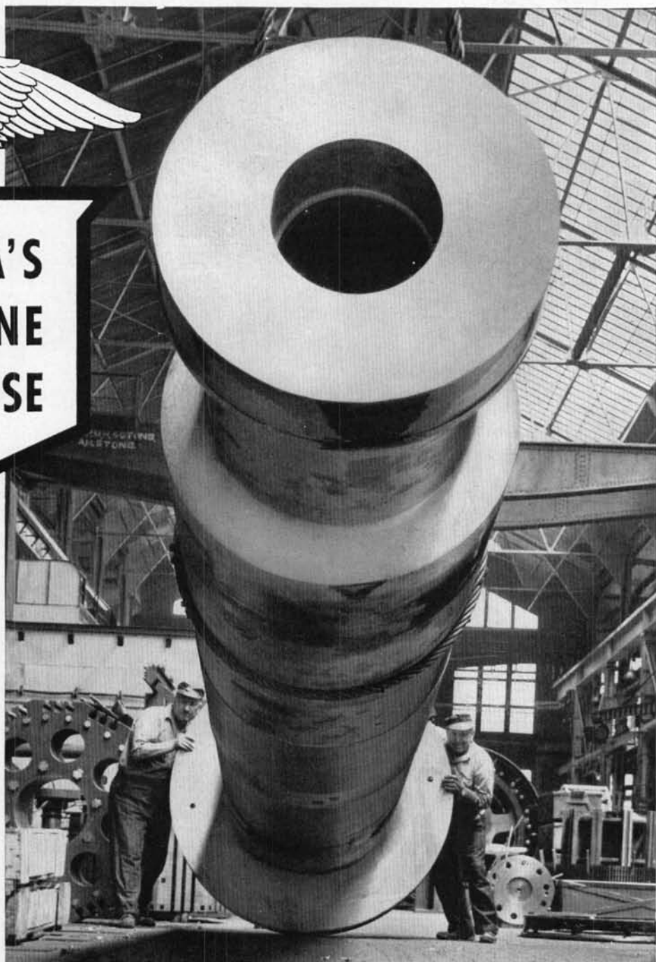
Not a cannon, but the 130,000-pound shaft for a great electric generator being built in the General Electric shops in Schenectady. When completed, the generator will deliver 75,000 horsepower of electricity.
