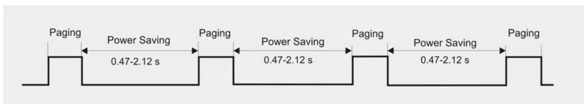
Figure 9: Power saving and paging in GSM networks
