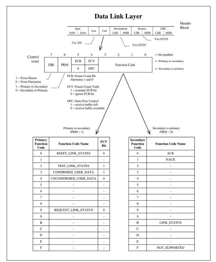
Figure 1 - Data link layer header breakout
