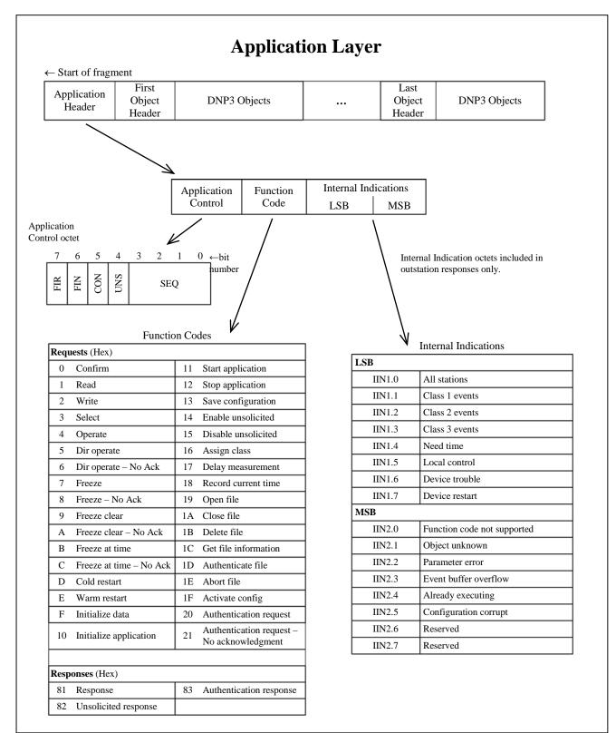
Figure 3 - Application layer header breakout
