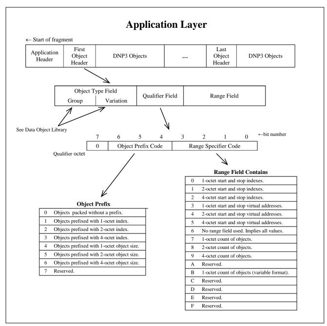
Figure 4 - Object header breakout
