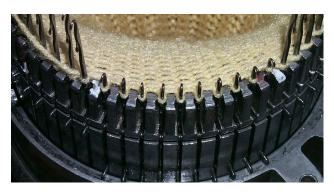
The final pass should be from left to right, with the yarn carrier stopping at the back. If you use the heel hook, now is the time to insert it into the work. When placed, you can see the pull on the stitches near the ½ marks. Hold down on the heel hook, at the same time use the other hand to reach up into the cylinder and check that the hook points are not hanging by one strand of yarn; hang a weight from the hook.
