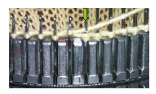
On your last pass, left to right, stop with the yarn carrier at the front and push down the two remaining needles on each side and all of the back needles (latches open!).
