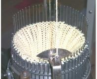
3. Knit around to the back until the tops of the working cylinder needles are level. Raise the last cylinder needle at the
