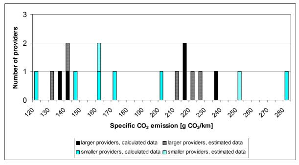
**Fig. 3.4:** Specific  $CO_2$  emission of light-duty vehicles in the Car-Sharing fleet (n = 18)
