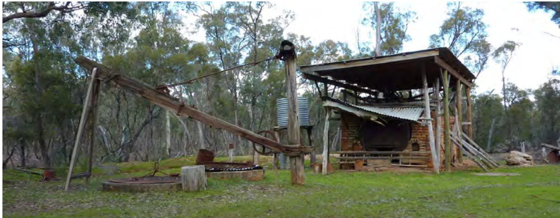
From left: Crane derrick, with brick vats below, and boiler in brick housing at right.
