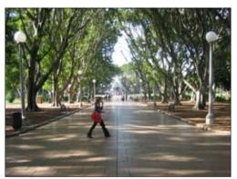
MAIN AVENUES Width: 8.6 metres Paving: Granite unit paver Kerb & Gutter: Pre-cast concrete
