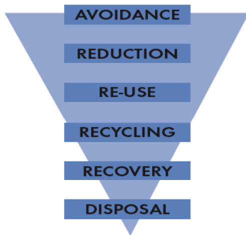
Figure 1 - Hierarchy for waste management. Source: A Waste Management Strategy for Canberra: No Waste by 2010, 1996, p8
