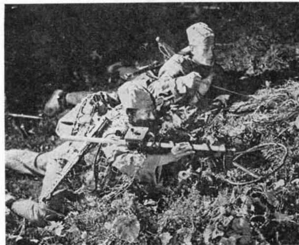
Figure 102. Soviet Mine Detector, VIM-203.
