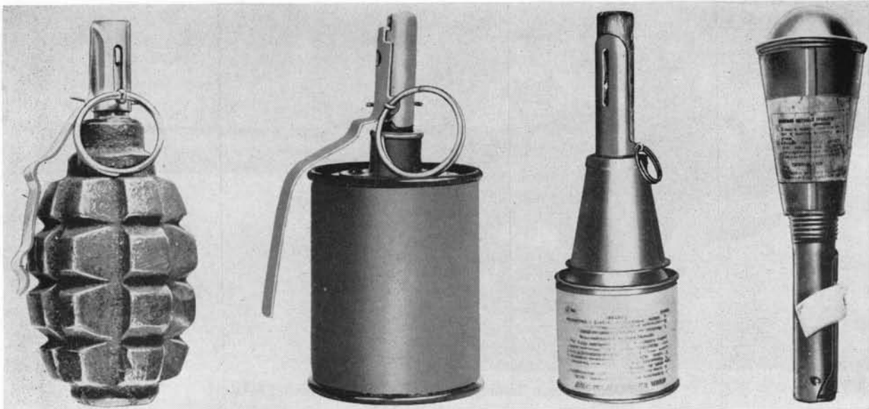
Figure 72. F-1 Defensive Hand Grenade, RG-42 Offensive Hand Grenade, RPG-43 and RPG-6 Heat Hand Grenades (left to right).
