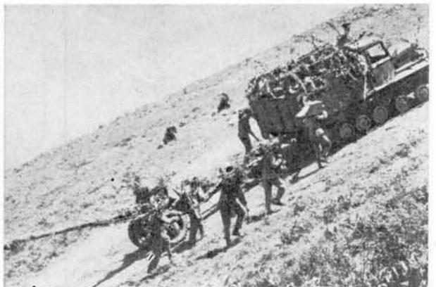
Figure 133. K-800 Prime Mover Towing 85-mm Gun.
