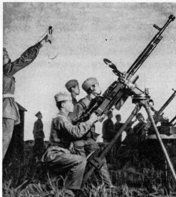
Figure 63. Chinese Communist 12.7-mm Heavy Machinegun, Type 54 (Soviet DShK, M1938/46).
