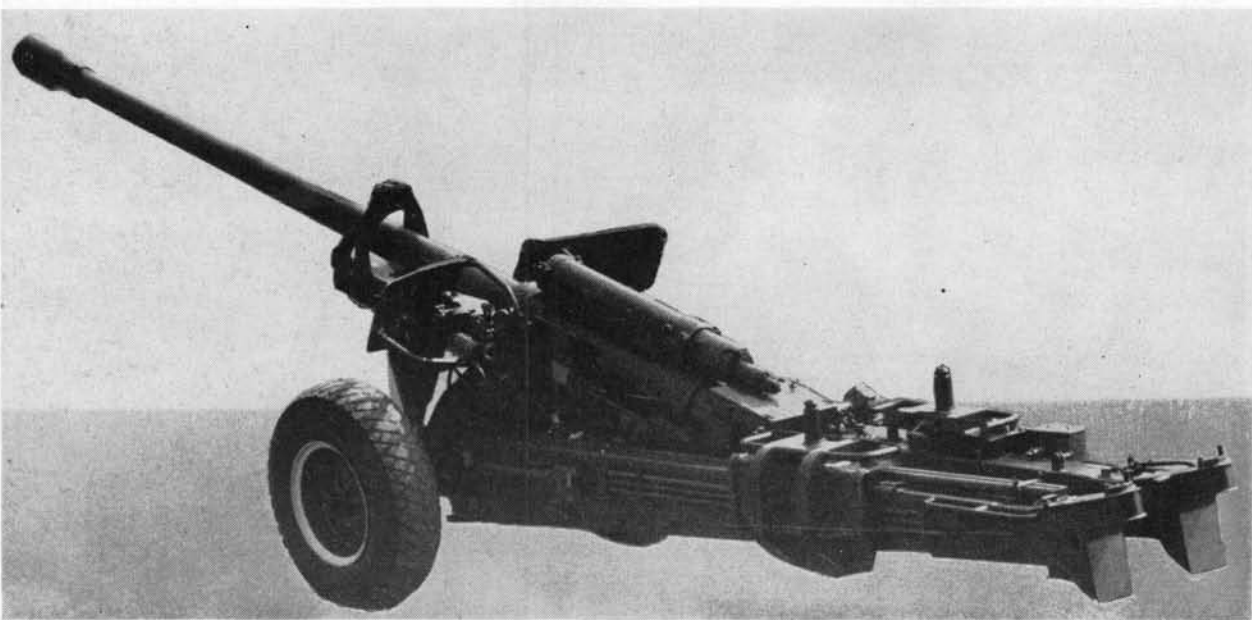
Figure 77. Soviet 130-mm Gun, M-46.
