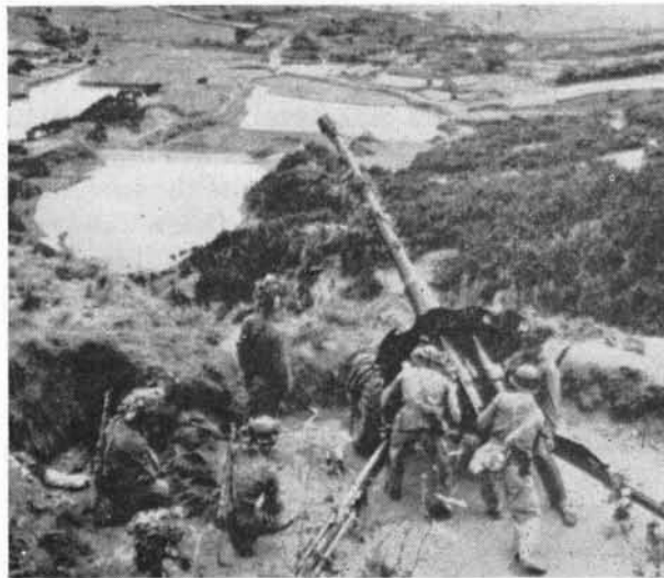
Figure 73. Soviet 85-mm Field Gun, D-44.
