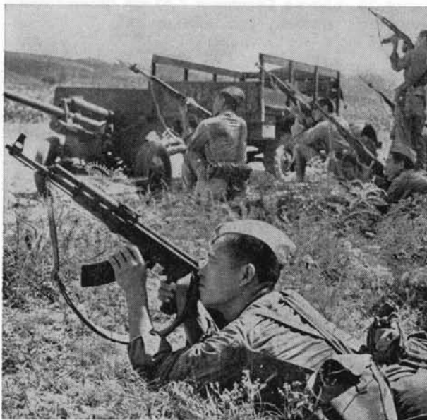
Figure 55. Chinese Communist 7.62-mm Submachinegun, Type 56 (Soviet AK) in Foreground. Chinese Communist 7.62-mm Carbine, Type 56 (Soviet SKS) in Background.
