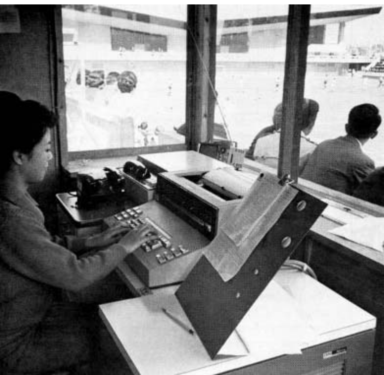
Data were transferred by data printers like these, to the printers in the Press Centre (right)
