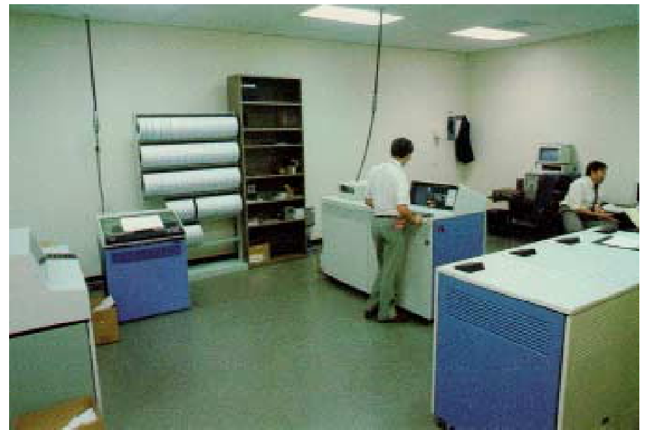
3 The LAOOC's computer ticketing needs are filled by two IBM System/38 computers at the LAOOC Ticket Data Center in downtown Los Angeles.
