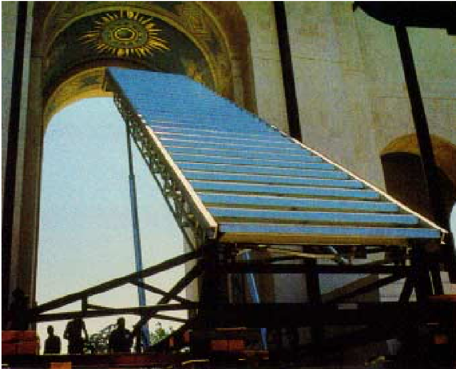
3 The hydraulic slip-stair used by the final torchbearer to light the torch is tested.
