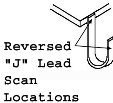
FIGURE 2037-4. Scan Locations on Reversed J-Style lead.
