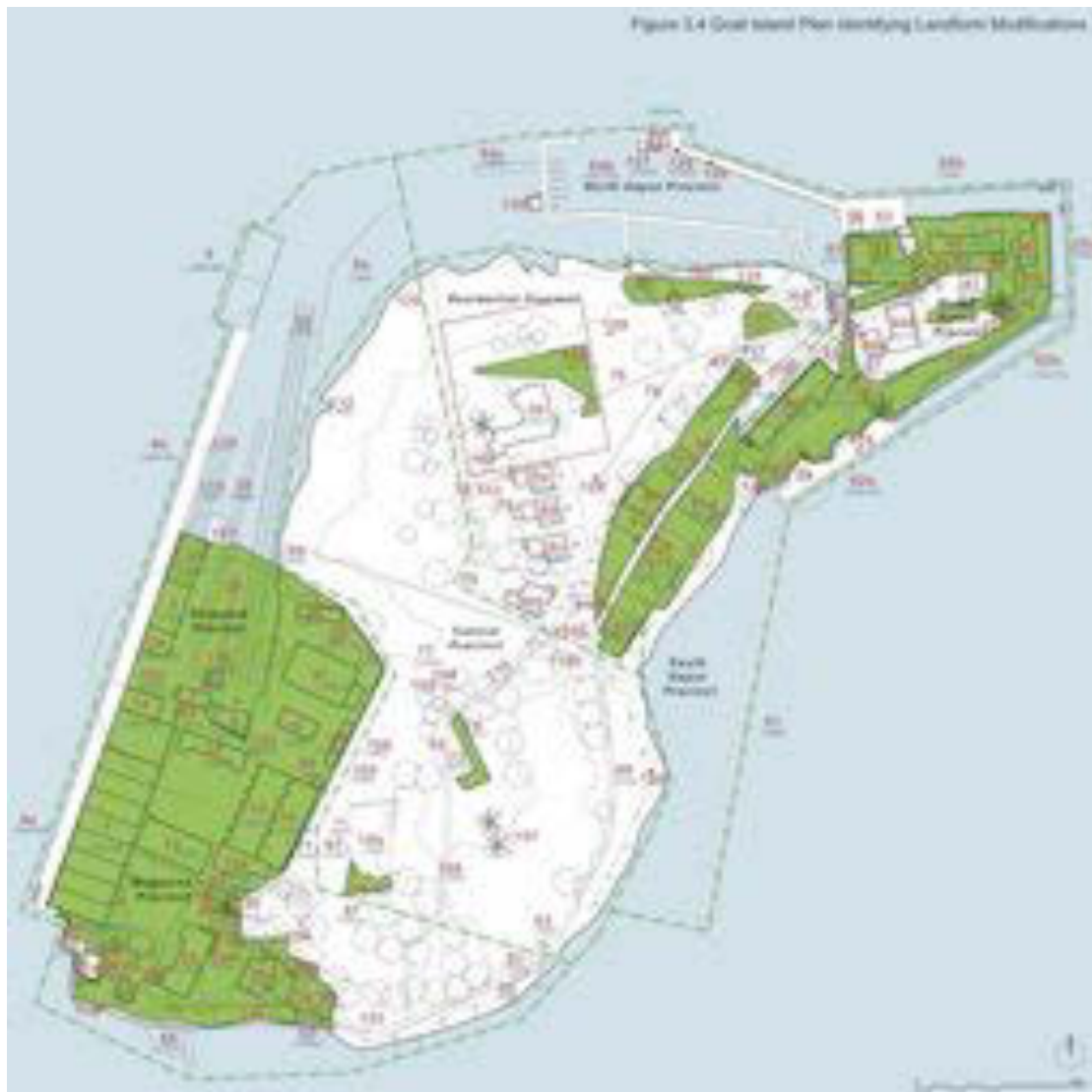
Figure 3.4 Plan of Goat island showing Areas of landform modification. The areas shaded green on the plan are the sections of the island that have undergone substantial landform modification through either quarrying and excavation and or fill including foreshore reclamation and cut and fill to create building platforms. Minor landform changes are not indicated. This plan is based on the 2007 aerial photograph and it is noted that sections of wharfs 4a, 4b, 5 and 51 and wharves 52b, 54c, 55a and 55b have collapsed and been removed.
