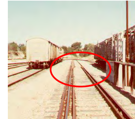
Transition: (3 gauge - centreline) for end wagon sheep transfer to (3 gauge common rail) for platform alignment (not visible)
