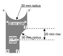
**4.2.** Gauge 2, Impact zone gauge, 100 mm radius, must be used to measure in plan sections AA' to BB' (front) and EE' to FF' (back).
