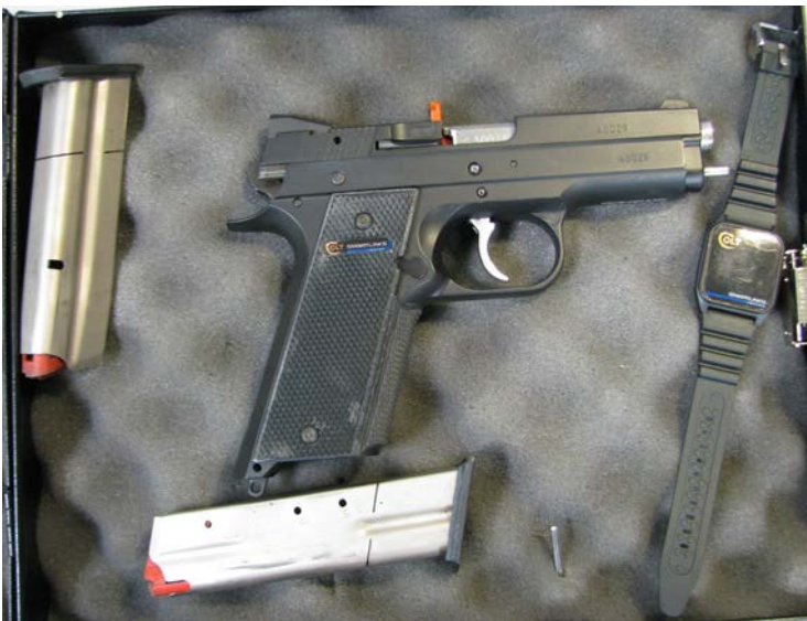
Figure 3. First of two Colt EP2 prototypes developed with SmartLinks and built on the .40 caliber CZ platform and delivered to NIJ.
