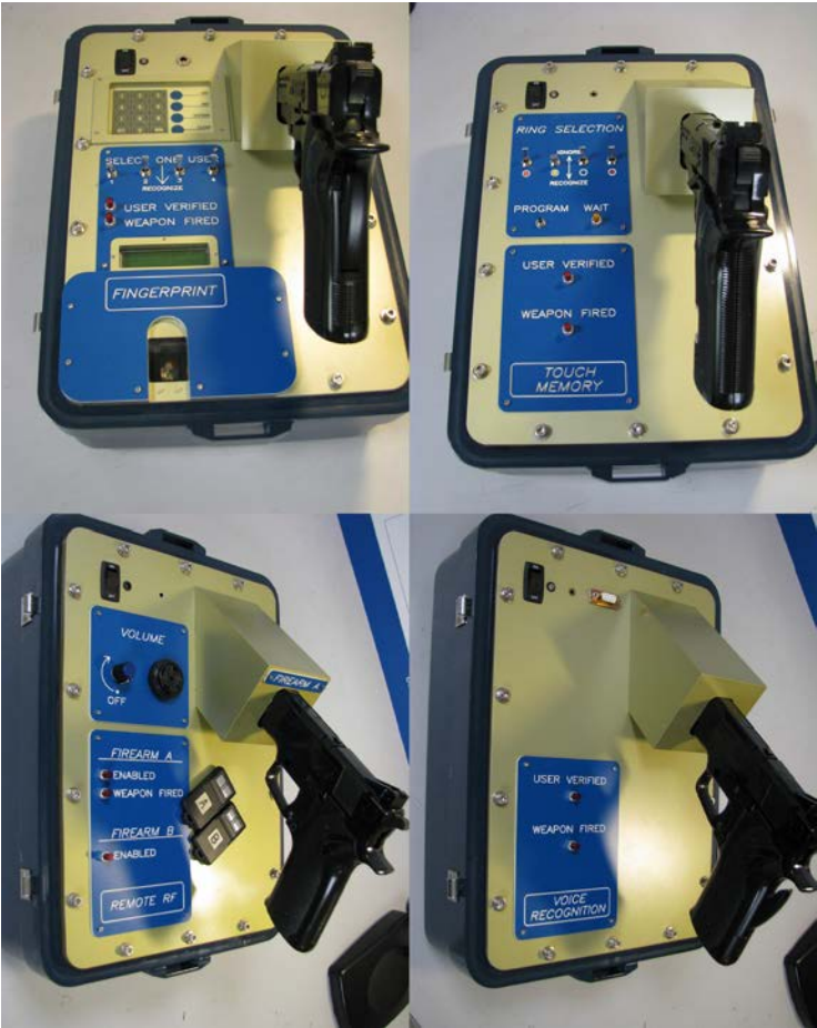
Figure 1. Various demonstrators produced by Sandia National Laboratories to illustrate the basic functionality of user authorization technologies, such as fingerprint (upper left), touch memory (upper right), remote RF (lower left), and voice recognition (lower right).
