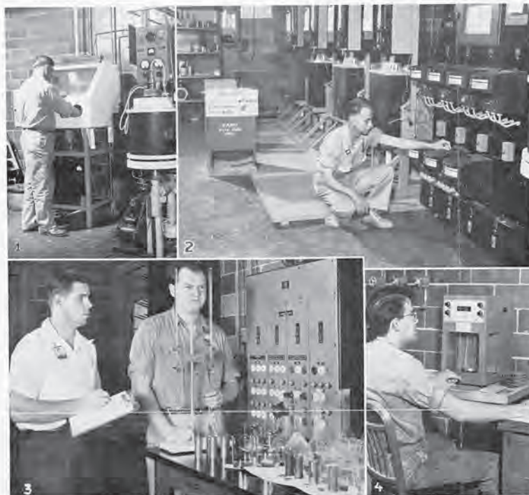
LIQUID METALS PROJECT REQUIRES MANY TECHNIQUES —(1) Technician James E. Pope places his hands in the rubber gloves built into the dry box and fills one of the toothpaste-tube medium and a tiny metal specimen preparatory to its being placed in a furnace of argon or helium to keep water and oxygen out. (2) With the specimen Proops sets the temperature controller on one of the eight furnaces used in the project. Shown are the four globar tube furnaces in which the hot zone is two and a half inches long. (3) Now ready for the stripping operation, the specimen is freed from which is titrated to determine the total amount of sodium or lithium that is Metallurgist L. A. Abrams, left, and Technician J. R. White is making the changes of the specimen on a gram-atic balance is Technician R. S. Webb. (4) The solid metal has dissolved into the sodium solution, or that some of the specimen.
