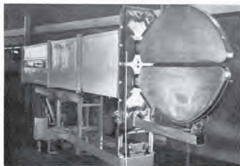
NEW ORNL CYCLOTRON MAKES NEWS —The 63-inch cyclotron at Y-12, operated by the Electromagnetic Research Division of Oak Ridge National Laboratory, is shown above. The cyclotron's "dees" (see story) are mounted in a vertical position and the whole system rests upon a motorized truck. Nitrogen ions originating in the ion source (not shown) placed in the center of the dees spiral outward until they strike the target, which is placed in the upper dee. When the deflector in the lower dee is used, the ions are directed into a target at the top of the vacuum chamber in which the dees operate. (Photo by Sienknecht)
