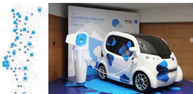
Fig. 23.3 MOBI.E vehicle electrification project includes installing charging stations in 30 municipalities and along main highways in its pilot phase, as well as developing an 80-km-range battery-electric vehicle, Mobicar, primarily aimed at the export market. (Image courtesy of MOBI.E)
