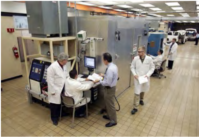
Fig. 10.1 Accelerated testing of Li-ion batteries. (Image courtesy of NREL.)
