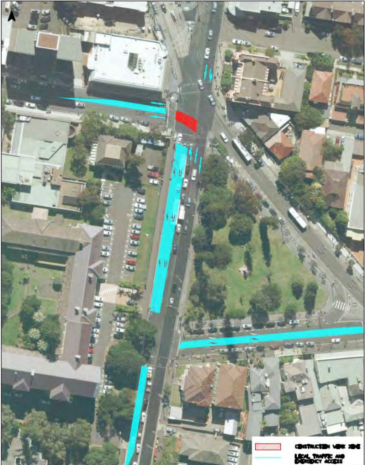
CSELR Belmore Street Crossover Staged Construction 2 of 3 (6 weekends total) Source: LPA 2011 APR 2013 60239638
