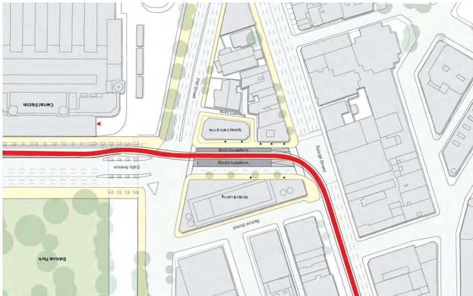
Figure 5-4: Light rail alignment along Rawson Place corridor
