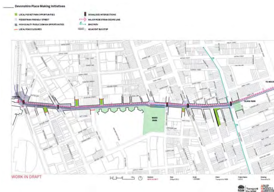
Figure 5-8: Light rail alignment along Devonshire Street corridor
