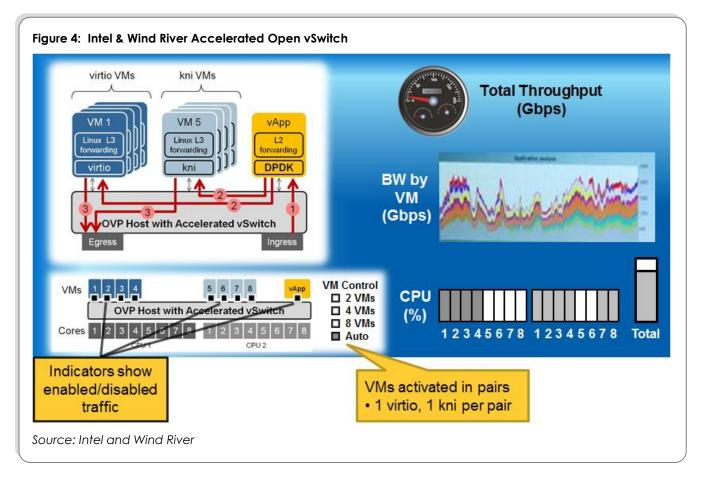
Intel and Wind River use a shared memory model, so that when packets come in the vSwitch analyzes the header and does not have to copy the packet. The vSwitch passes a pointer to get better overall performance.
