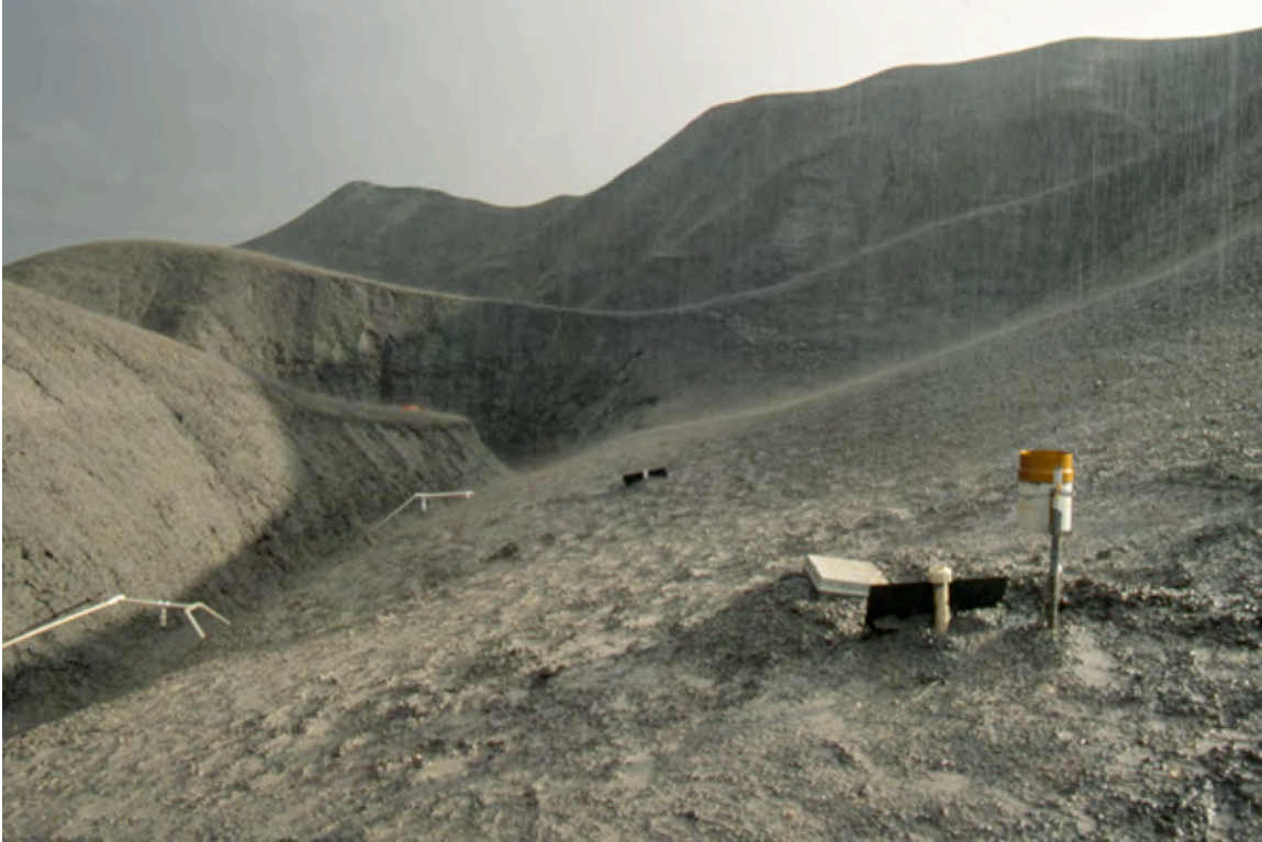
Downpour in Blue Hills badlands near Caineville, Utah. Raingage in the foreground records rainfall intensity, R , while PVC supports center sonic rangers over channel to record stage of resulting flashfloods.
