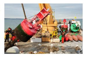
Lake Erie – The crew of Coast Guard Cutter BRISTOL BAY, removing a buoy in Nov 2012 as part of District 9's annual "Fall Retrieve", which is designed to limit damage to AToN in the winter months.
