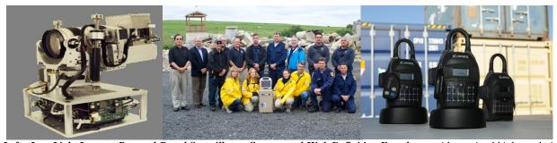
Left: Low Light Internet Protocol-Based Surveillance Camera and High Definition Encoder provides optimal high-resolution footage in a variety of lighting conditions and enables law enforcement to capture, compress, send, and encode video over a low bandwidth IP network in low light environments.
