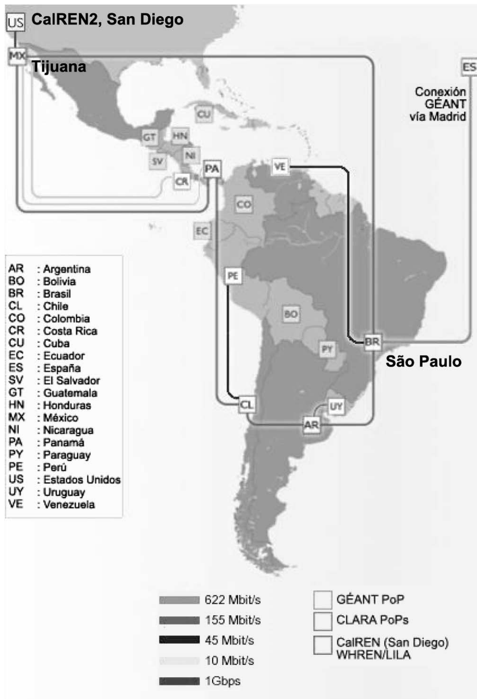
Fig. 4. Topology of CLARA Network showing performance bandwidths Points of Presence (PoPs) including the 155 Mbps connection between São Paulo, Brazil to Tijuana, Mexico and then the 1 Gbps connection to CalREN2 in San Diego. Courtesy of Latin American Cooperation of Advanced Networks, redCLARA, www.redclara.net .
