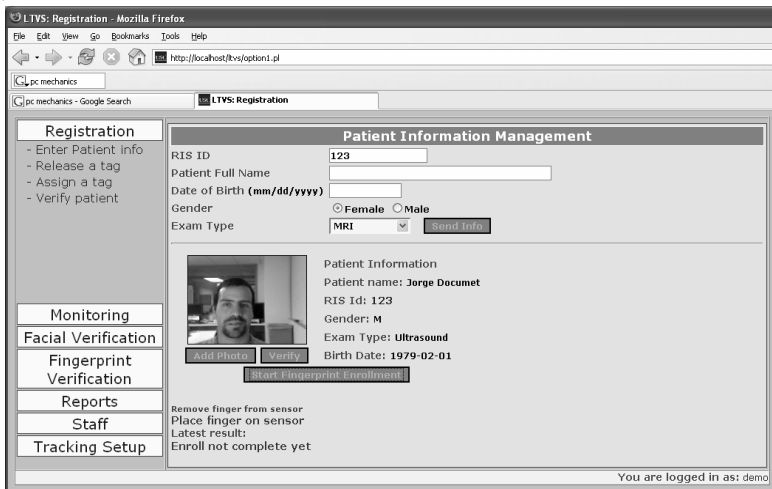
Figure 4- Patient registration page shows how to register a new patient into the LTVS system. First, a patient photo was captured by the video camera, correlated with patient information. After patient photo registration, the fingerprint enrollment step started by a system message says "Place finger on sensor".
