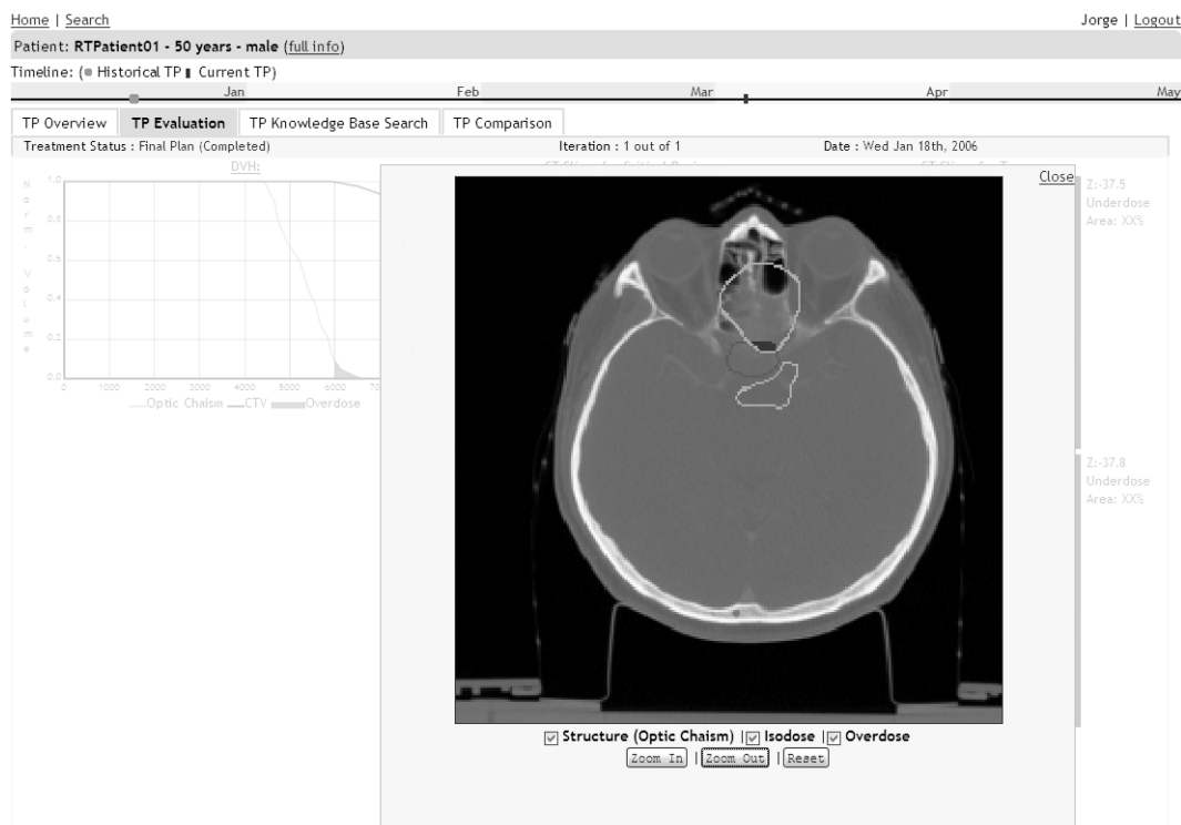
Fig. 9 Pop-Up Window Allowing the User to View the Area of Overdose to the Optic Chiasm in Greater Detail as Shown by the Arrow Pointing at the Shaded Region. The Optic Chiasm Region is outlined in gray while the specific percentage dose Isodose Curve that overlaps with Optic Chiasm Region producing Overdose or “Hot Spots” is outlined in White. Note that there are two separate Isodose Curves where there is a specific percentage dose, which shows that the treatment plan is attempting to avoid Radiation Dose to the Optic Chiasm Region. Even so, there is still overdose as indicated by this particular screen shot and the shaded region highlighted
