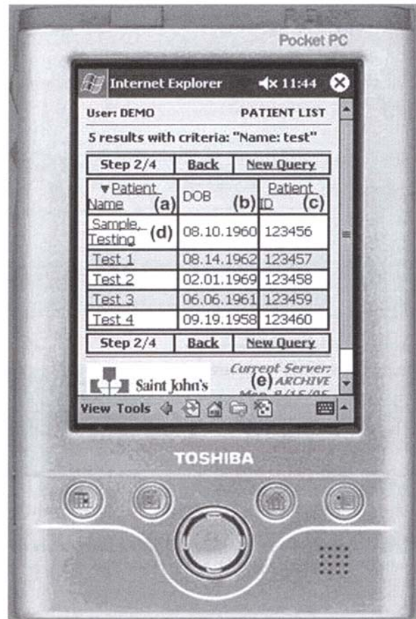
Fig 3. Step 2: this screen shows the list of patients who matched the input search criteria from the previous step. The user can sort the results by using either "patient name" (a) or "patient ID" (c). The date of birth (b) is also shown as a reference but is not sortable. To obtain the list of studies for a particular patient, the user can tab the patient name of any of the results. In this example, the patient "Testing, Sample" (d) is selected. Field (e) shows the current server from which the query was obtained.
