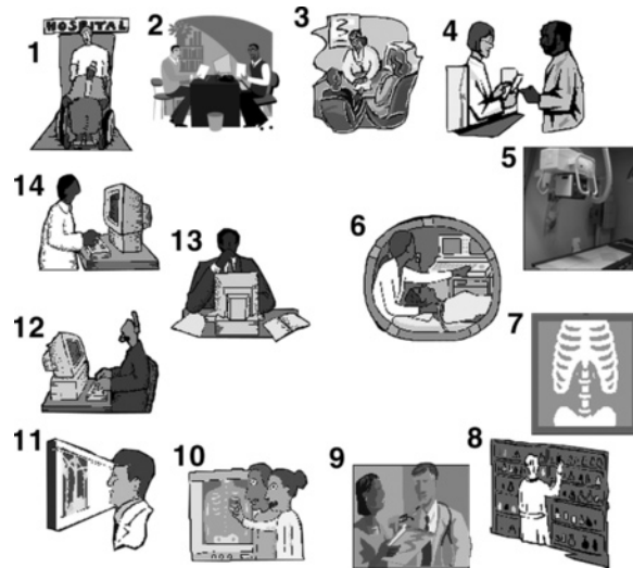
Figure 1. Chart illustrates the impact of a PACS on clinical work flow in a radiology department. Step 1, patient arrives at hospital; step 2, patient registers with hospital information system; step 3, examination is ordered at radiology information system; step 4, technologist receives information from clerk; step 5, patient is escorted into modality room; step 6, technologist performs examination; step 7, examination is completed; step 8, clerk pulls out old films; step 9, clerk prepares all necessary papers and films for radiologist; step 10, films are hung up for radiologist's review; step 11, radiologist reviews films, reads examinations, and dictates reports; step 12, transcriptionist types draft report from the dictation; step 13, radiologist reviews and signs off on report; step 14, final reports are input into radiology information system for clinical viewing. With the implementation of a PACS, steps 4, 8–10, 12, and 14 can be eliminated, making work flow more efficient. (Modified, with permission, from reference 3.)
