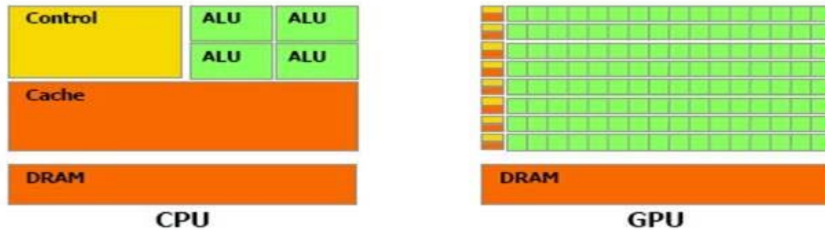
Figure 1. The difference in CPU and GPU architecture (ALU: Arithmetic Logic Unit)
